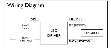
Input and Output use lead-wires. Lead-wires are 20AWG 80C/300V stranded copper
